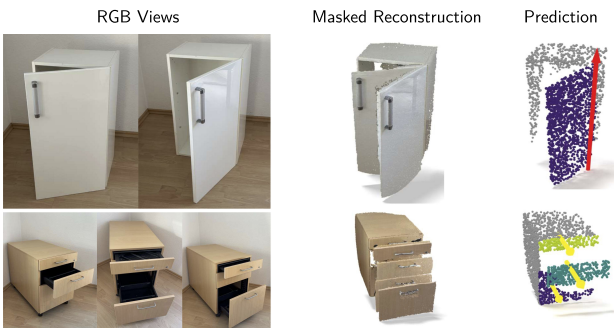
Figure 6. Real-world objects. Masks are obtained with SAM2 [45] and reconstruction with VGGT- \Omega [53]. Despite being trained only on synthetic data, FAMOS generalizes to casual real-world captures.
